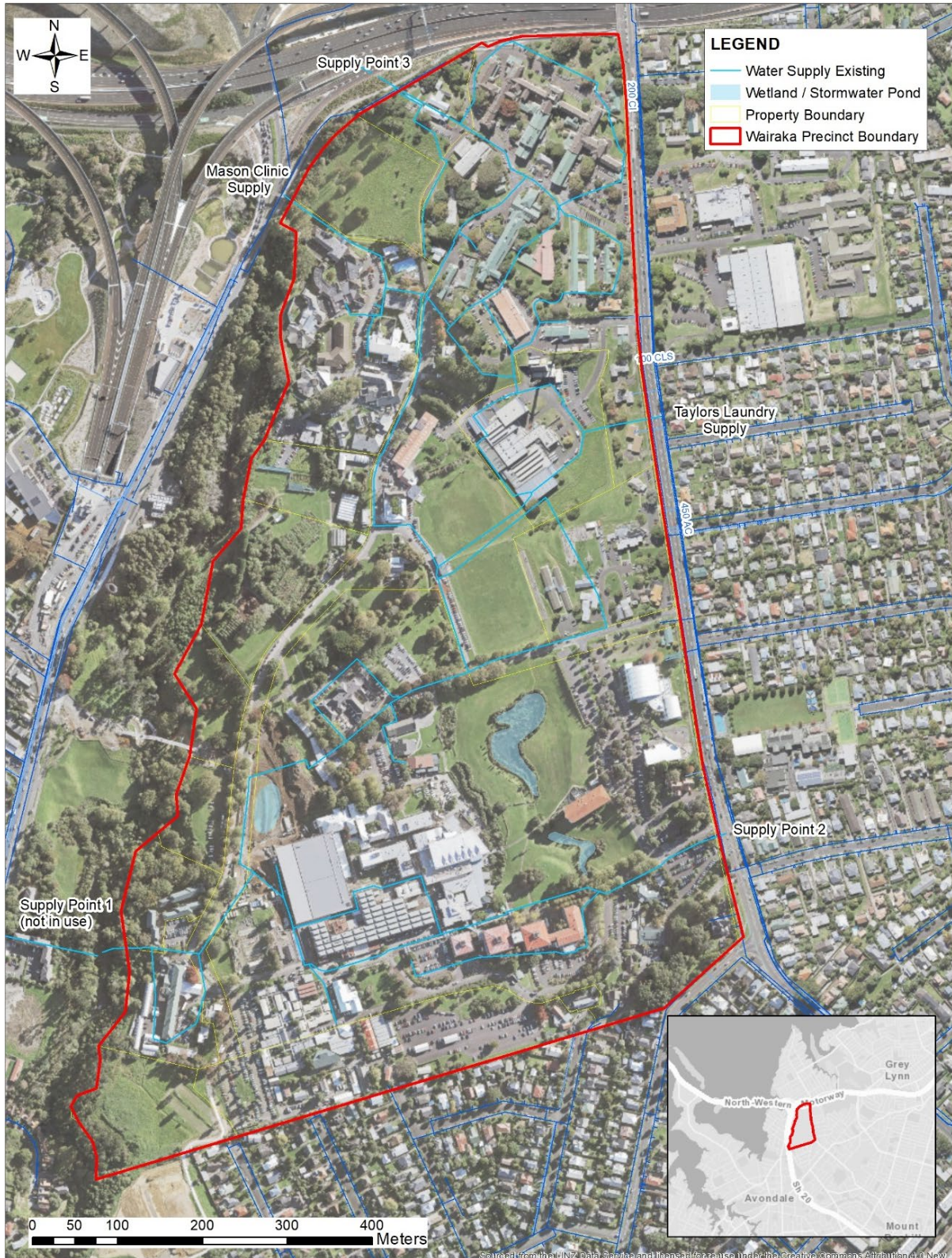
Figure 8 Existing Water Supply System
