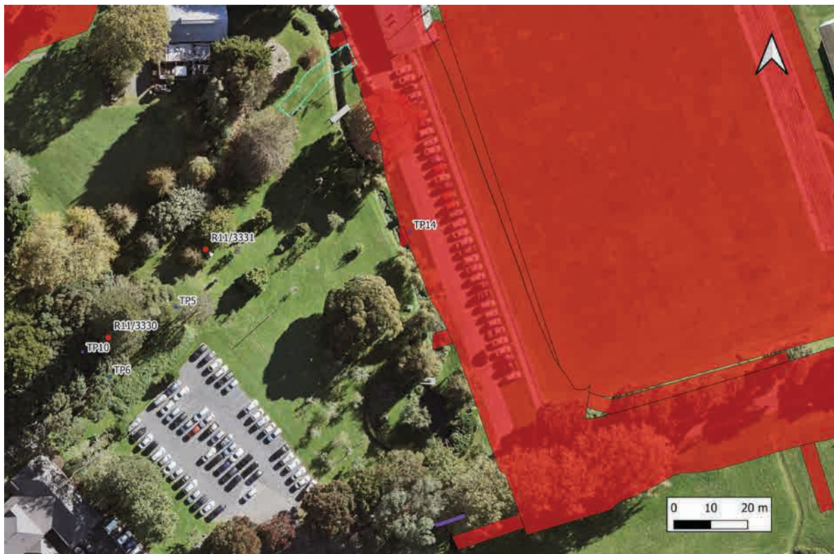
Figure 14. Location of stormwater trenching from proposed Farm Road into Wairaka Stream (red area) in relation to existing stone culvert (purple), original driveway to farm manager's house (light blue dashed).
